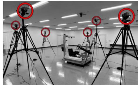
Fig.9 Position of the Motion Capture Cameras
