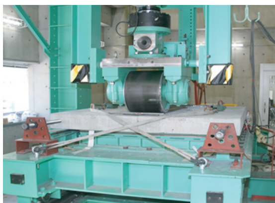
PIC. 2 Wheel-running fatigue test unit
