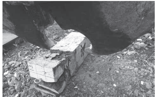
Fig. 13 A beam specimen of W/C=13% after repeated crushing loads showing the shortage of the crushing power
