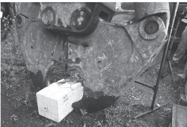
Fig. 11 A specimen held with the attachment
