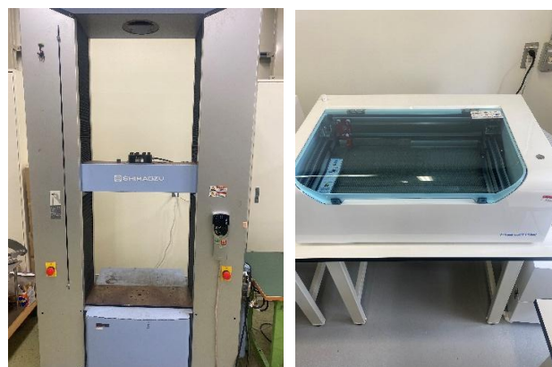
a) Tensile testing machine b) Laser processing machine
