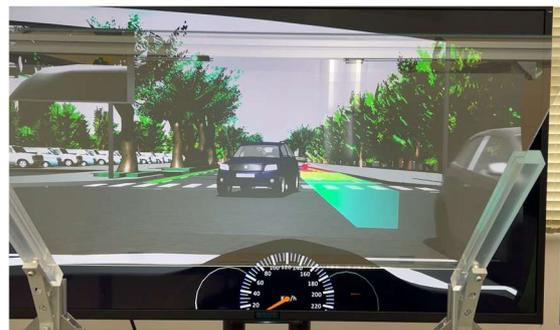
Fig. 4 Image of space margin indication on road surface
