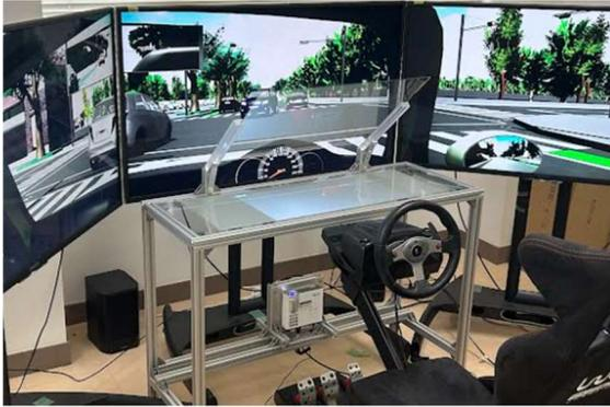
Fig. 1 Overview of fixed-base driving simulator
