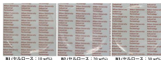
Fig. 5 Fabricated cellulose-PEG film materials.
