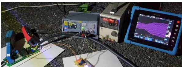
Fig.3 Charging power step response experiment on Honda e
