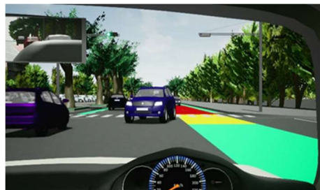
Fig. 1 Image of space margin indication on road surface
