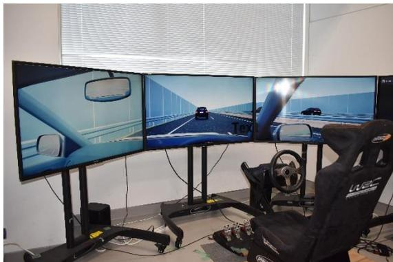
Fig. 5 Overview of driving simulator
