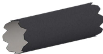
Fig.1 FRP cylinder model with slit.
