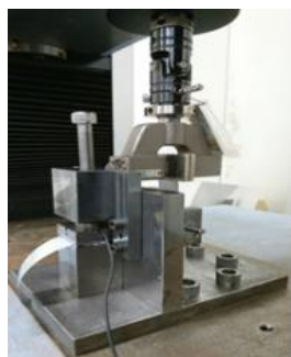
Fig.2-2 Friction test jig
