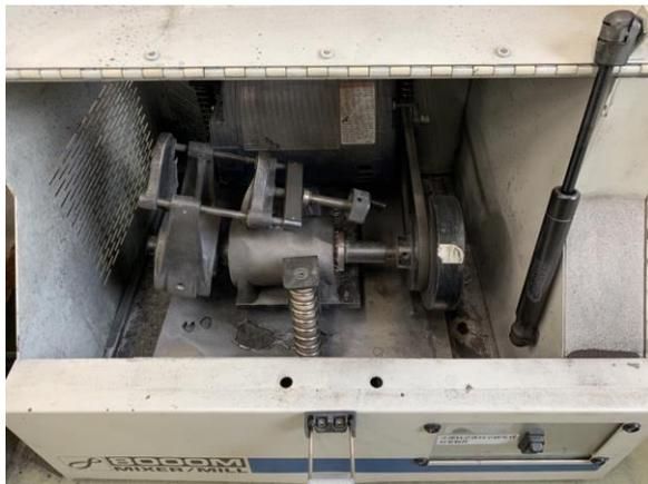
Fig. 3 Appearance of vibratory ball mill
