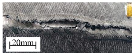
Fig.7 Burst part of type B
