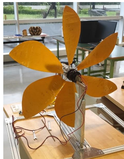
Fig.7 Wind turbine considering tip loss factor
