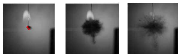
(b) Micro-explosion of a n-Hexadecane/water emulsion droplet by Phantom Miro310
