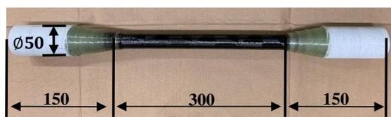
Fig.2 Specimen for torsional test (unit:mm)
