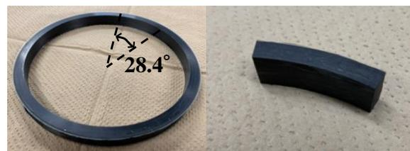
(a) CFRP ring (b) Specimen
