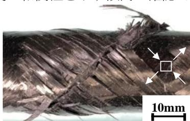
Fig.3 Type B shaft after failure
