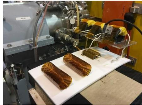
Figure 7: RFKO system prototype (WERC's electrode).
