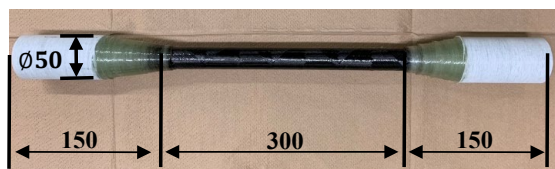
Fig.3 Specimen for torsional test (unit:mm)
