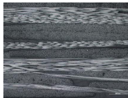
Fig.1 Observation of cross section for urethane CFRTP.
