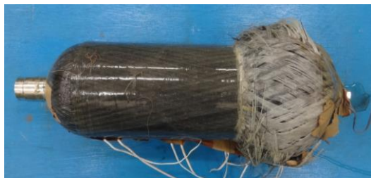
Fig.3 No.1 Type4 vessel after burst test
