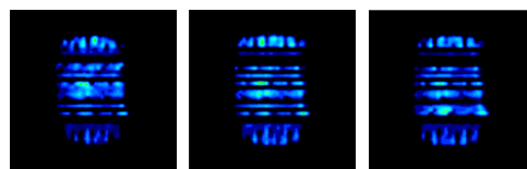
Fig.5 Contact pressure of Front-Right tire on Sports
