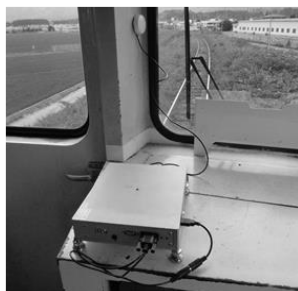
Fig.3 Measurement of car-body acceleration using on-board sensing device
