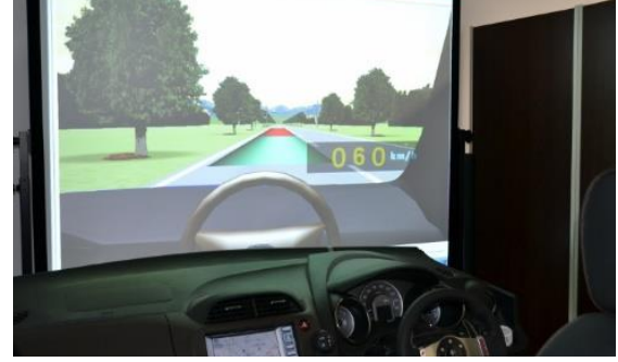
Fig. 2 Overview of fixed-base driving simulator
