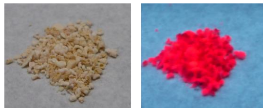
Fig.3 Photographs of red-emitting \text{Na}_3\text{AlF}_6:\text{Mn}^{4+} phosphor. (Excitation lamp: 302 \text{ nm} )
