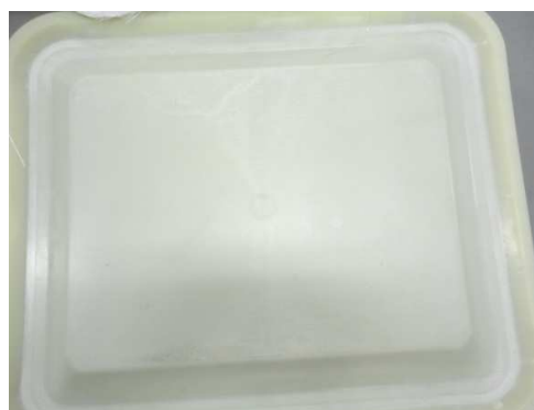
Fig.2 GFRTP using in-situ polymerizable PA6
