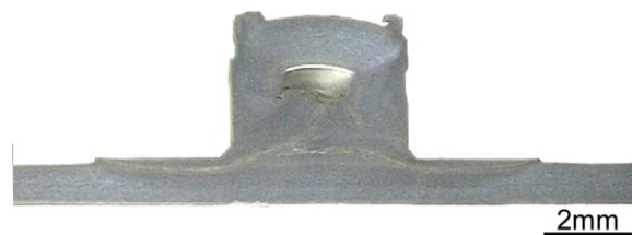
Fig.4 Macrostructure of protrusion. ( d = \phi 10\text{mm} , N=1500\text{rpm} )
