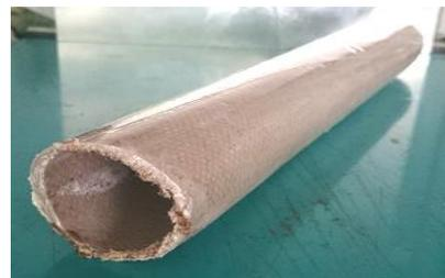
Fig.5 Cylindrical shell made of green composite
