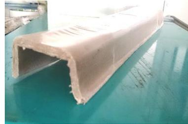
Fig.4 Channel made of green composite
