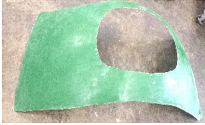
Fig.2 Roof part made of green composite.
