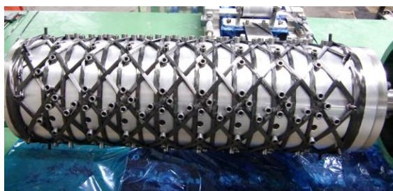
Fig.1 Fabrication of cylindrical CFRP grid by using a guide pin type mandrel.
