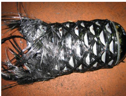
Fig.4 CFRP grids pressure vessel after burst test.
