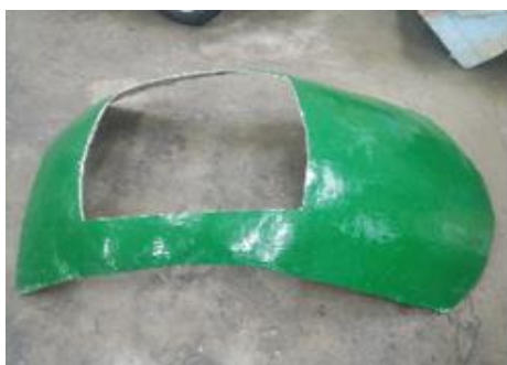
Fig.4 Roof part made of green composite
