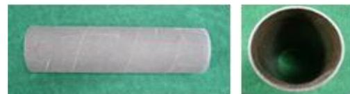
Fig. 4 A cylindrical shell PBS/LINEN
