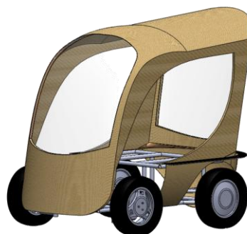
Fig.9 Design of body shell made of green composite
