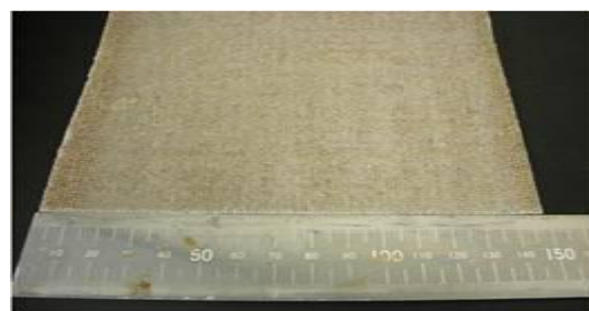
Fig. 2 PBS/LINEN Pultrusion material
