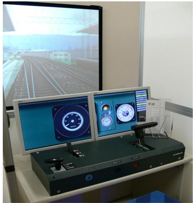
Fig.4 Overview of train-driving simulator
