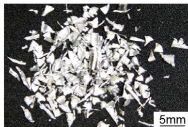
Fig.1 Appearance of 6063 aluminum alloy chip.
