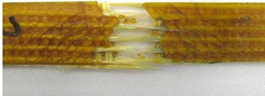
Fig.10 Fracture surfaces of with coating
