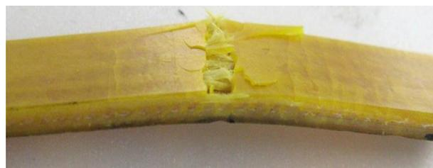
Fig.12 Fracture surfaces of with coating
