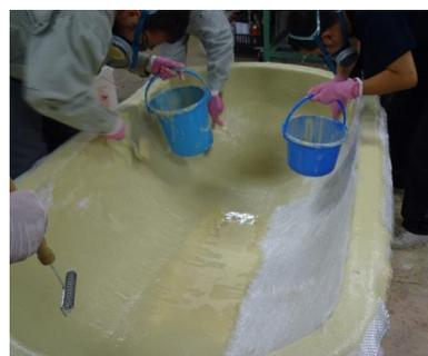
Fig.1 Hand lay-up process
