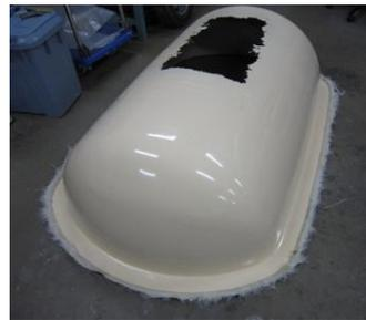
Fig.2 Upper body shell before trimming
