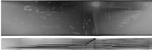
Fig.2 X-ray Inspection (t=3.1mm Delamination Area 658mm<sup>2</sup>)
