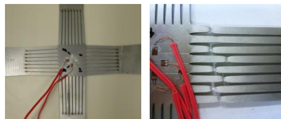
(a) The middle of test (b) After a test Fig.4 Specimen in the middle and after test
