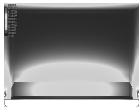
Fig. 6.2 Illuminance Distribution (With Light-shelf The spring and autumnal equinox 12:00 Fine)
