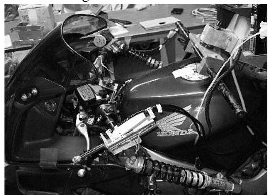
Fig.2 Sub-Steering System
