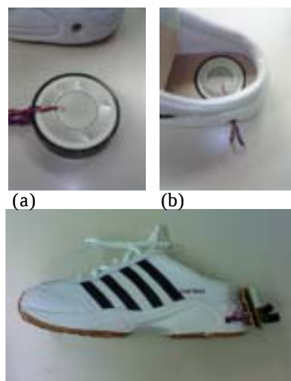
Fig.8 Piezo cell installed in a shoe
