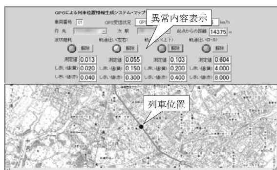
Fig. 11 Display of Fault and Position on a Map
