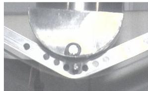
Fig.7 Delamination of adhesion layer.
