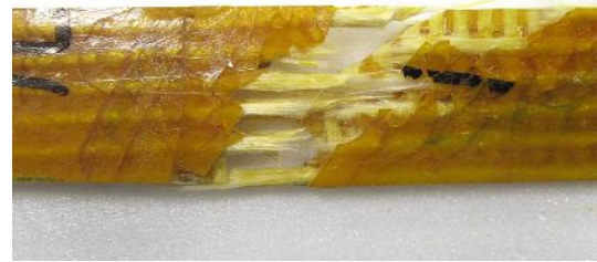
Fig.9 Fracture Surfaces (A)
