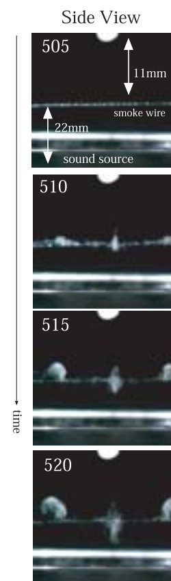
Fig. 5 Pictures showing the diffusion of fine paraffin particles. Each frame is in time interval of 5ms.
