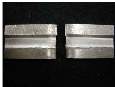
Fig.5 Specimen after U-bending test. (FSW0° , Face side)
