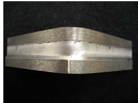
Fig.3 Specimen after V-bending test. (FSW0° , Face side)
