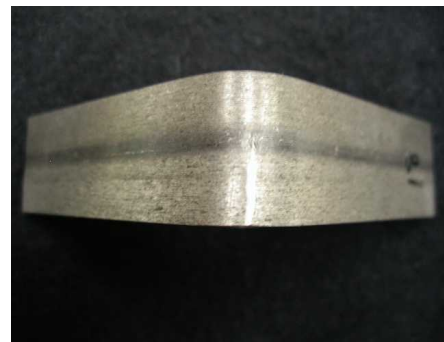
Fig.4 Specimen after V-bending test. (FSW0° , Root side)
