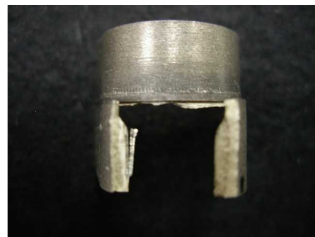
Fig.6 Specimen after U-bending test. (FSW0° , Root side)
