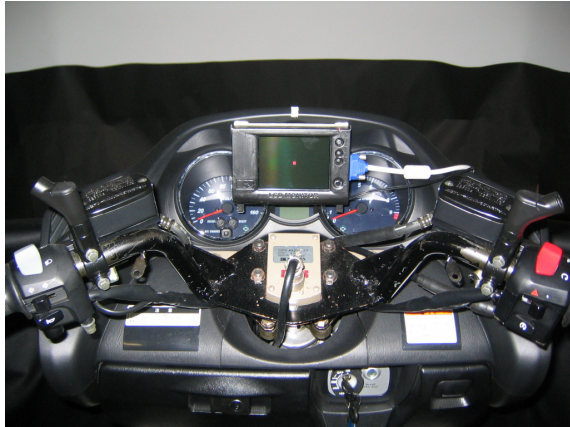
Fig.7 Real-time parameter tuning system for Rider
