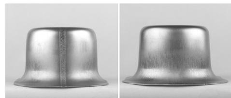
Fig.13 Side view of deep drawing tested specimen.
