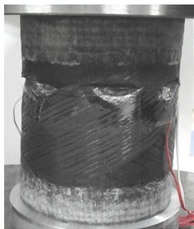
Fig.14 Buckling Deformation of Isogrid60° Cylindrical Shell
