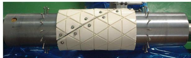
Fig.3 Mandrel Covered with Silicon Rubber Mold
