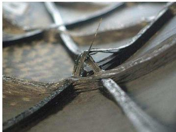
Fig.13 Failure at Offset Point (Isogrid90° Cylindrical Shell)
