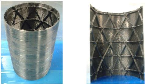
Fig.5 Whole and Half Section of Cured Isogrid Cylindrical Shell
