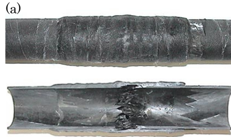
Fig. 9 Failure Aspect of the Specimen (50mm, 20Pieces) (a) Appearance, (b) Cut Section
